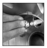
After mounting the spare, put the wheel nuts back on with the rounded end of the nuts toward the wheel. Tighten each wheel nut by hand.
